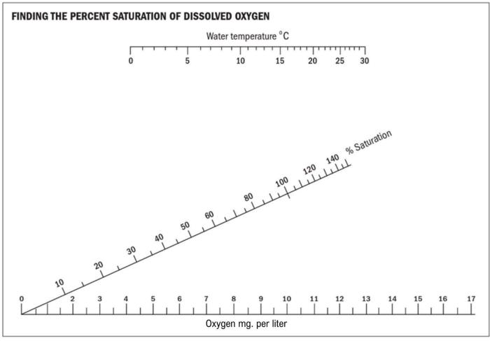
To read this chart, use a straight edge. Place the straight edge on the mg/L of oxygen you have determined for your site, then place the other end of the straight edge on the water temperature you have measured. The point where the straight line passes through the line labeled "% Saturation" is your percent saturation.
