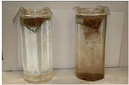
Figure 53. In the slake test, dried chunks of soil from fields under different management are suspended in columns of water. Soil from fields managed with reduced tillage and other healthy soils practices remains intact for long periods in water ( left ), while unhealthy soil from conventionally tilled fields quickly falls apart in water because the soil structure has been damaged ( right ). This simple test is a compelling visual illustration of how no-till reduces erosion. Source: NRCS.
