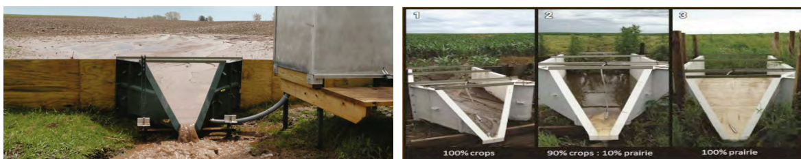
Figure 45. Left: Water streaming off a flooded field that has been tilled, illustrating the magnitude of sediment loss from water erosion in tilled fields left fallow. NRCS; Photo credit: USGS. Right: These flumes measure surface water movement and nutrient concentrations in runoff from experimental fields in Iowa containing different percentages of prairie plants. Even including a strip of prairie plants comprising only 10% of a corn or soybean field has a dramatic impact on the amount and quality of the water leaving the field. Source: Ref. 169.
