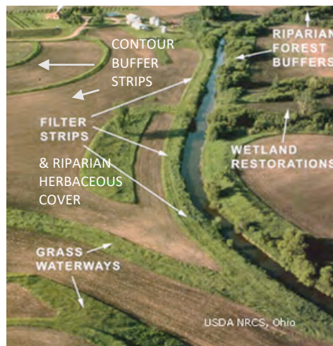
Figure 36. Examples of several practices involving herbaceous cover, showing how their placement can intercept or direct water to filter out chemicals & sediment and reduce erosion. Modified from USDA NRCS.
