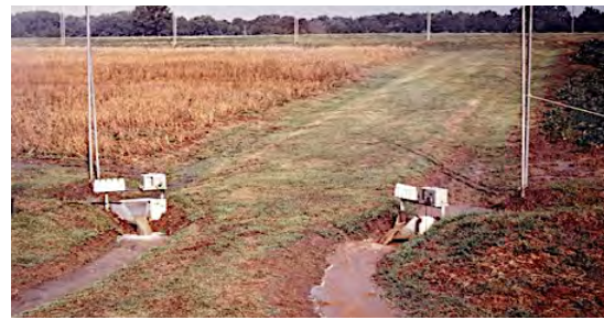
Figure 46. Demonstration of the impact of soil health practices on runoff quantity and sediment load. The field on the left was planted using no-till while the field on the right was conventionally tilled in the fall and left fallow over the winter. Runoff from the no-till field contained visibly less sediment than runoff from the conventionally managed field. Credit: Arnold King, NRCS.
